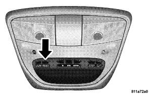
Use this button to reset the following displays to zero: Average Fuel Economy Trip Odometer Elapsed time.
